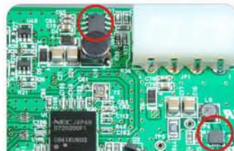
Switching power regulators for best stability
