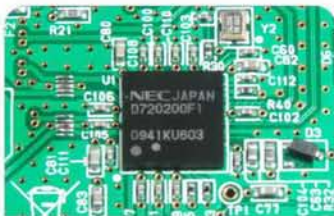
NEC \mu PD720200 chipset for best performance
