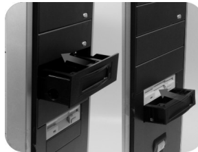
3.5" and 5.25" removable bays allowing for any type of installation in PC cases
